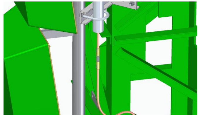
Figure 4. Detail of installation of the dinnteco connector.
